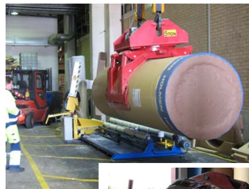
Loading – with overhead crane or clamp truck
