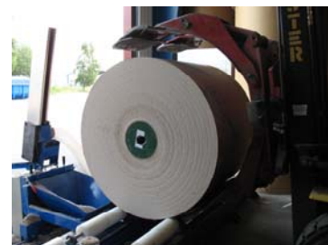
Loading – with overhead crane or clamp truck
